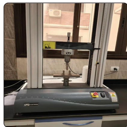
Fig. (2) Specimen in Universal testing machine for measuring flexural strength
