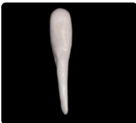
Fig. (2) Milled PEEK post with 10 mm in length.
