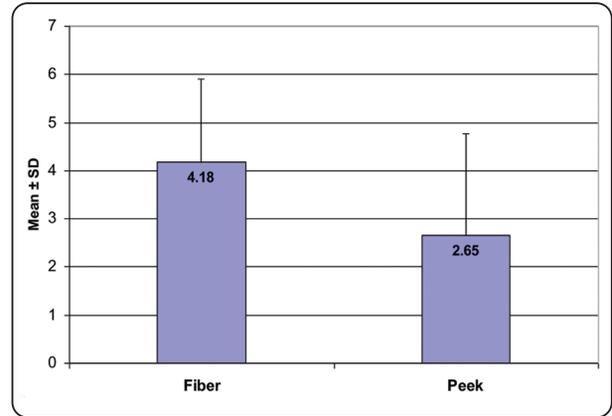
Fig. (7): Histogram presenting Push-out strength in each post type based on sections.
