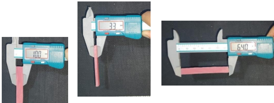
Fig.2: 3.3mm thickness, 64 mm length and 10 mm width are dimension of flexure strength test and hardness test specimens.
