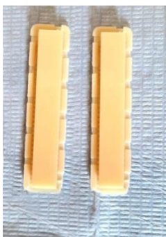
Fig.1: 3D printed model of the specimens
