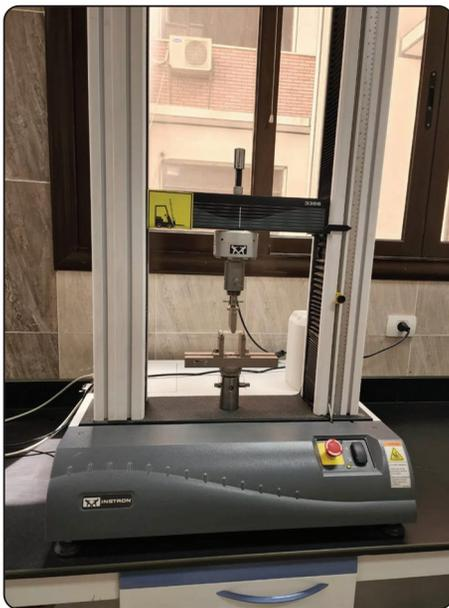
Fig. (2) Specimen in Universal testing machine for measuring flexural strength
