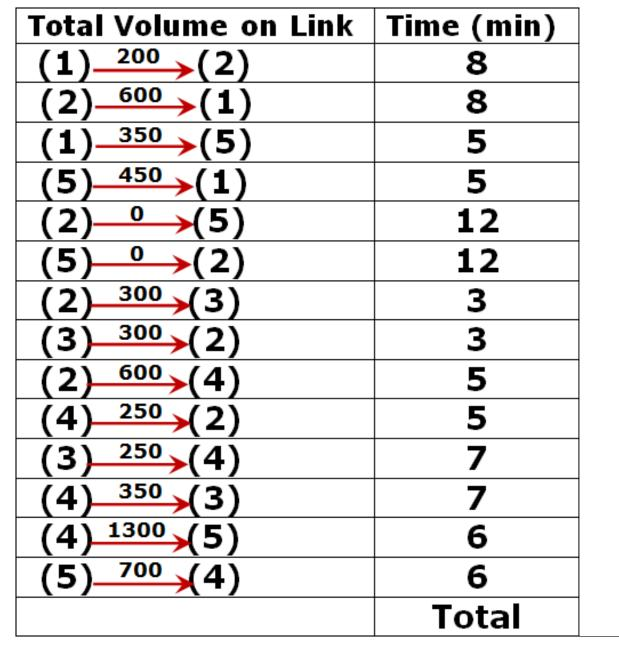
**Example**: The figure represents travel times on the link connecting six zonal centroids. Determine the minimum path from each zone to each other zone. Use the all-or-nothing assignment method to determine the total trips for each link after all of the trips from the following two-way trip table have been loaded onto the network.
