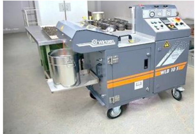
Fig. 8: Laboratory-Scale Foaming Device (WLB 10 S): Foaming Nozzle and Foaming Device [66], [67].
