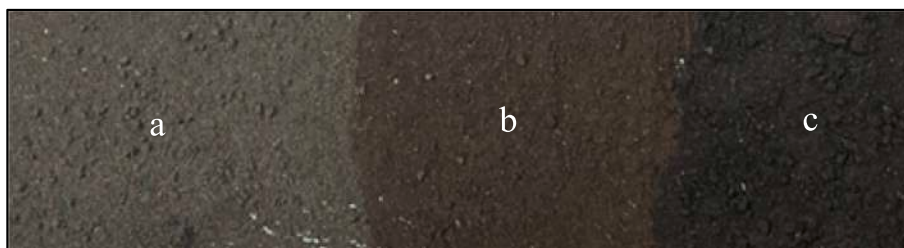
Fig. 4. Three separation products produced from the developed magnetic flotation system; (a) hydrophilic/non-magnetic product, (b) magnetic product, (c) floating product.
