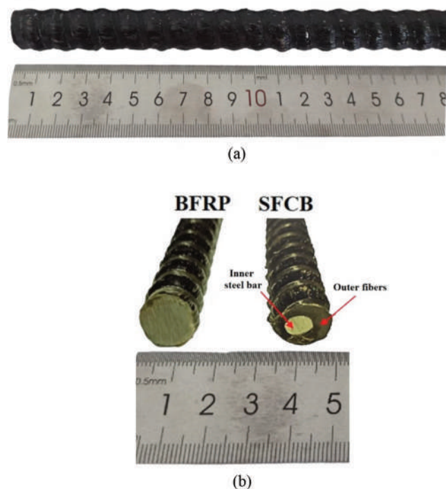
Fig. 1—Configuration of BFRP and SFCB reinforcing bars: (a) geometry of BFRP and SFCB bars; and (b) cross sections.
