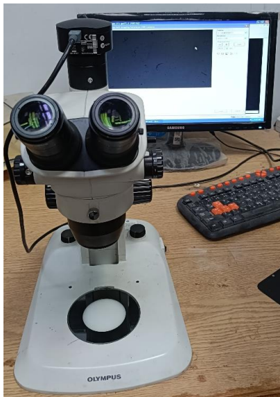
Fig. 5: Stereomicroscope to identify delamination
