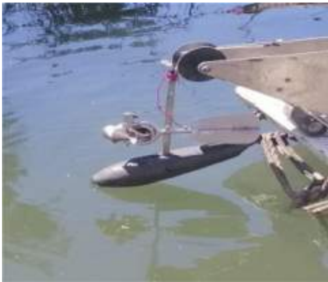
Fig. 7. The used current meter type G269.
