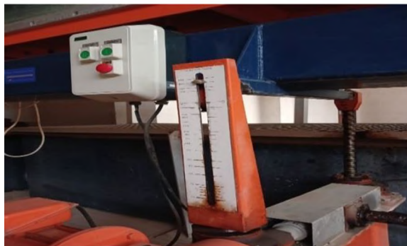
Photo (5): the gauge of the sloping channel
