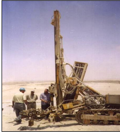
Figure (2): The Rotary drill machine used at Grawai Quarry
