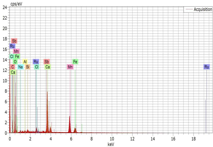
**Fig. (3) The EDS analysis showing the elemental composition of a typical mineral particle which is shown in Fig. (4).**
