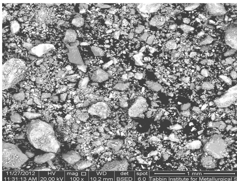
Fig. (2): A Back scattered scanning electron microscope (SEM) micrograph of a crushed sample
