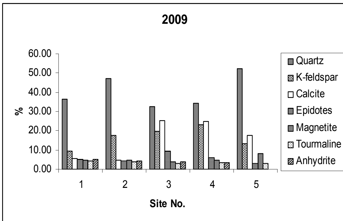
Figure 7: Distribution of common minerals in the sites of Khamasin dust samples in 2009 year
