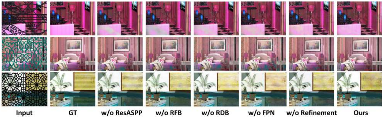
Fig. 11. Visual analysis of the ablation study, showcasing the influence of each model component on overall performance.
